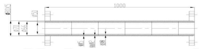
Ceramic 8mm + steel 5mm + glue 2mm
